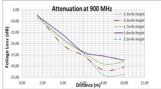
Figure 1 (Top) electrical field and (bottom) attenuation at 900MHz
