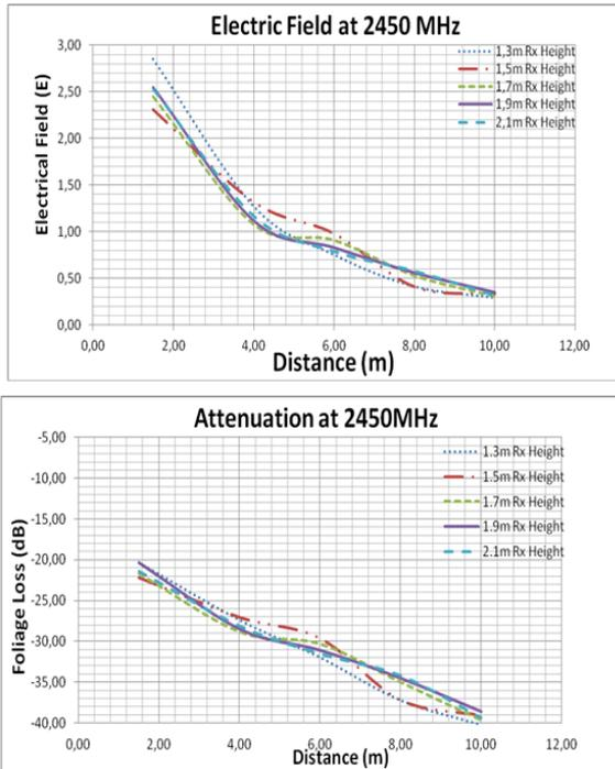
Figure 4 (Top) electrical field and (bottom) attenuation at 2450MHz
