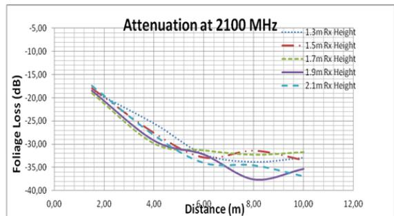
Figure 3 (Top) electrical field and (bottom) attenuation at 2100MHz
