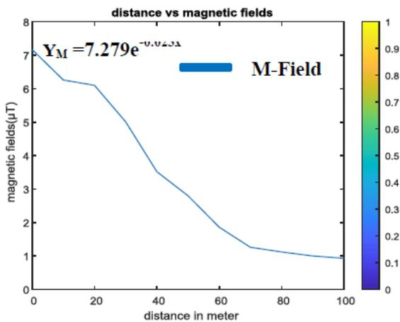
Figure 2b: Graph of the Magnetic fields from 330Kv power transmission lines at Ayede-Egbeda community as a function of horizontal distance.
