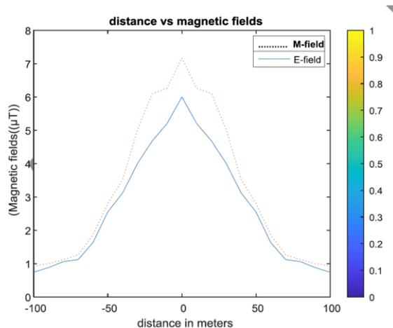
Figure 5: A graph of Magnetic fields generated under powerlines.
