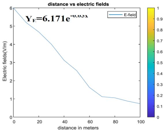
Figure 2a: Graph of the Electric fields from 330Kv power transmission lines at Ayede-Egbeda community as a function of horizontal distance.
