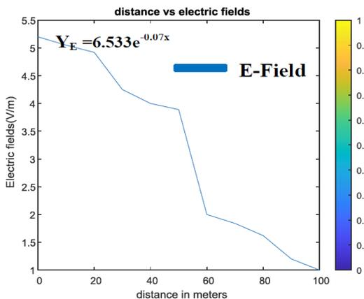
Figure 3a: Graph of the Electric fields from 132Kv power transmission lines at University of Ibadan as a function of horizontal distance.
