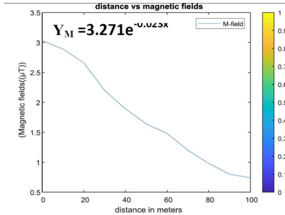
Figure 4b: Graph of the Magnetic fields from 33Kv power transmission lines at Shasha Ojoo as a functional distance.
