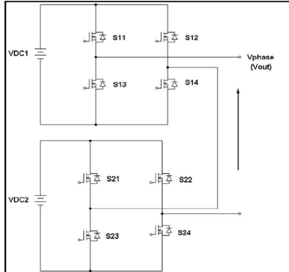
Fig 4. Single Phase Structure of Cascaded Five-level Inverter
