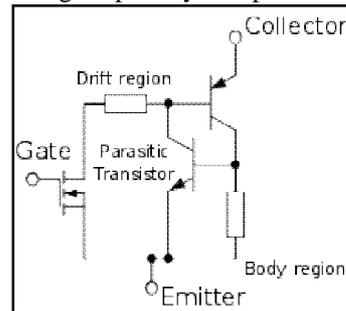
Fig 2. Equivalent circuit of IGBT
