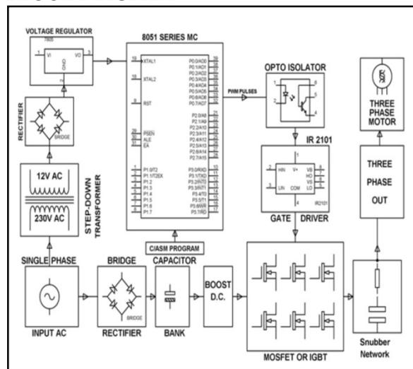
Fig 1. Block Diagram of the proposed scheme
