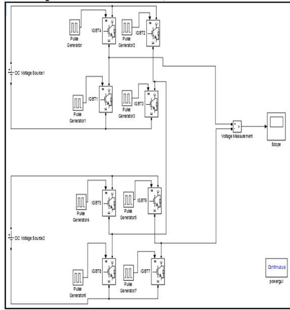
**Fig 7. MATLAB Simulation Diagram for 1-phase CHB Inverter**
