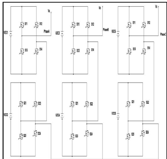
Fig 5. Three Phase Structure Of Cascaded Five- Level Inverter
