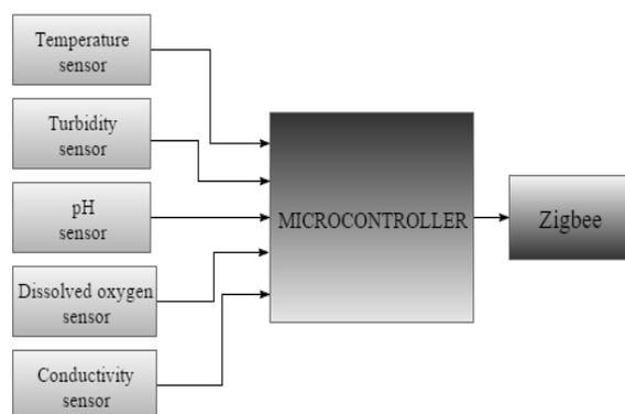
Fig.2. Block diagram of Device
